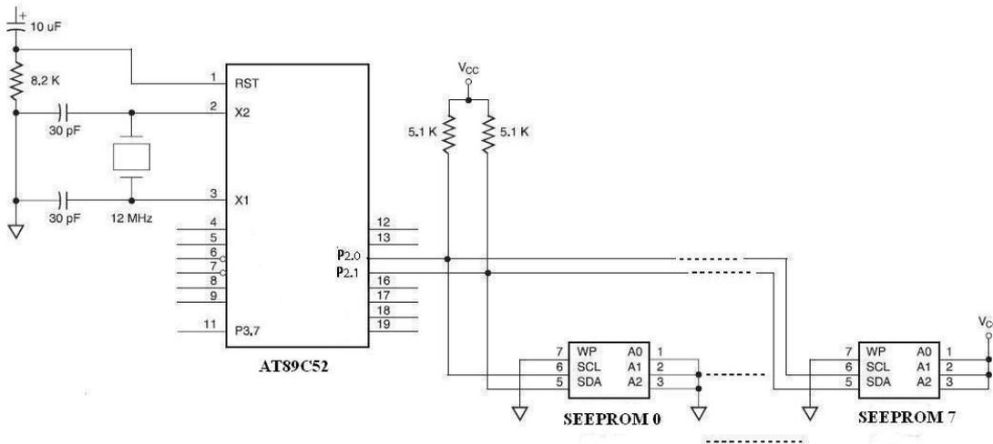
Figure 5 Multi Serial EEPROM( SEEPROM) interfacing
